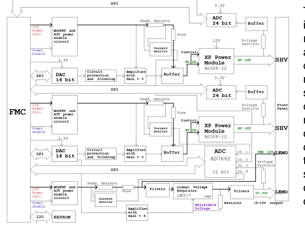
The high-voltage output is monitored by a highresolution ADC through 1:1000 high-voltage а divider. An auxiliary ADC measures the primary side of the HV DC/DC converter to indirectly the monitor power consumption the at output, and at the same allow time to a supervision algorithm to control power dissipation.
