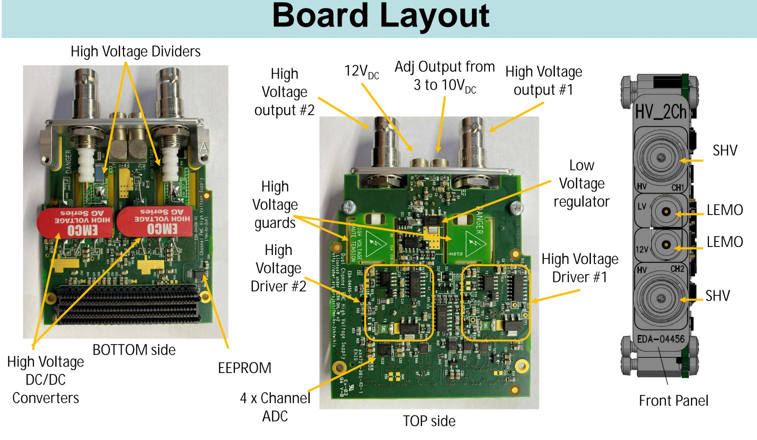
The PCB design required particular attention due to the presence of high-voltage, which is a potential source of safety issues, electrical discharges, and current leakage. For these reasons, dedicated high-voltage guards have been created on the PCB by applying the following rules:
