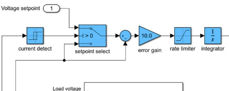
The algorithm is modelled with Matlab/Simulink to test the different strategies for the feedback controller. The left figure shows, as blue blocks, the feedback-based voltage and current controller topology that was selected. It is built around one integrator with a gain and a saturation to set the maximum voltage rate.
